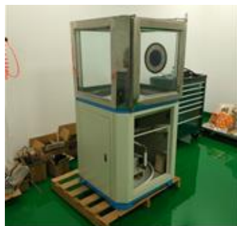
Figure 3 Humidity verification device
