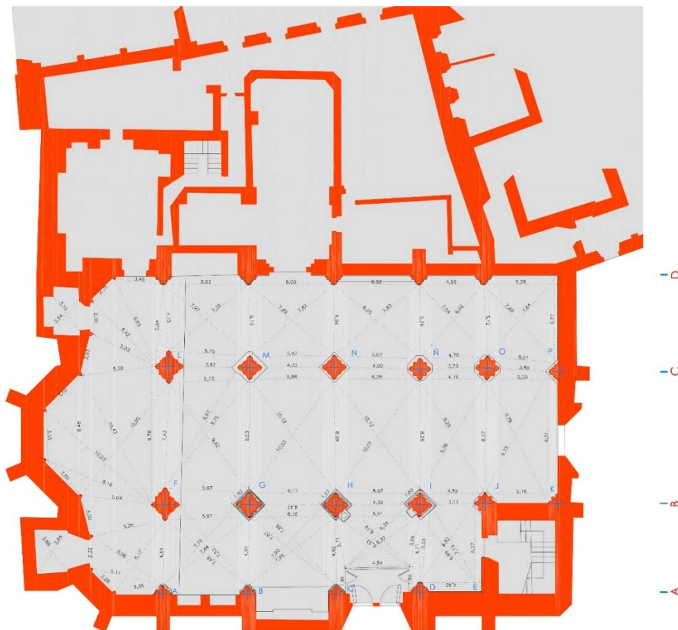
Figure 5. Plan of the Co-Cathedral of Santa Maria did with Photogrammetric method
