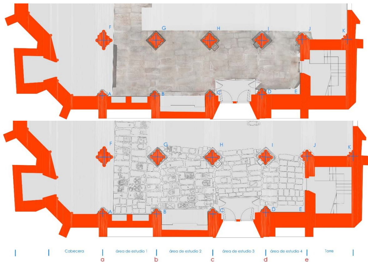
Figure 7. Photogrammetric method. Plane with images and plane to line derived from work
