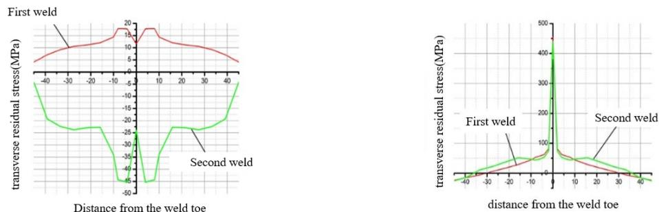
**Figure 4.** transverse residual stress comparison. **Figure 5.** longitudinal residual stress comparison.
