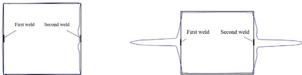
**Figure 2.** Transverse residual stress distribution. **Figure 3.** Longitudinal residual stress distribution.
