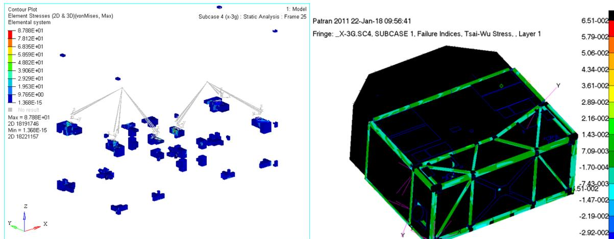
**Figure 6.** Cloud chart of stress distribution in titanium alloy joints and composite material failure indices by the Tsai-Wu criterion
