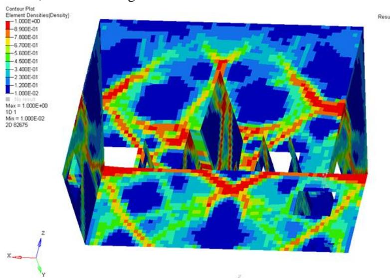
**Figure 1.** Optimization result for the main frame
