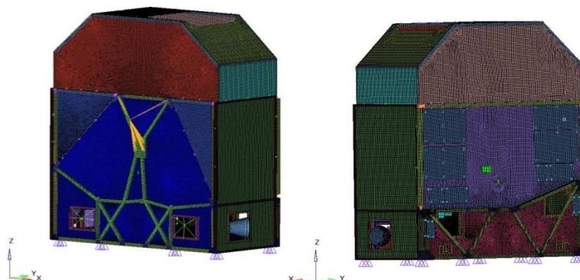
**Figure 3.** Finite element model of the mapping camera system
