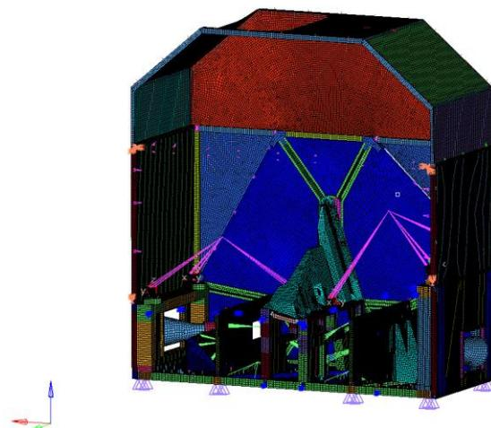
**Figure 5.** Finite element model of the mapping camera system.
