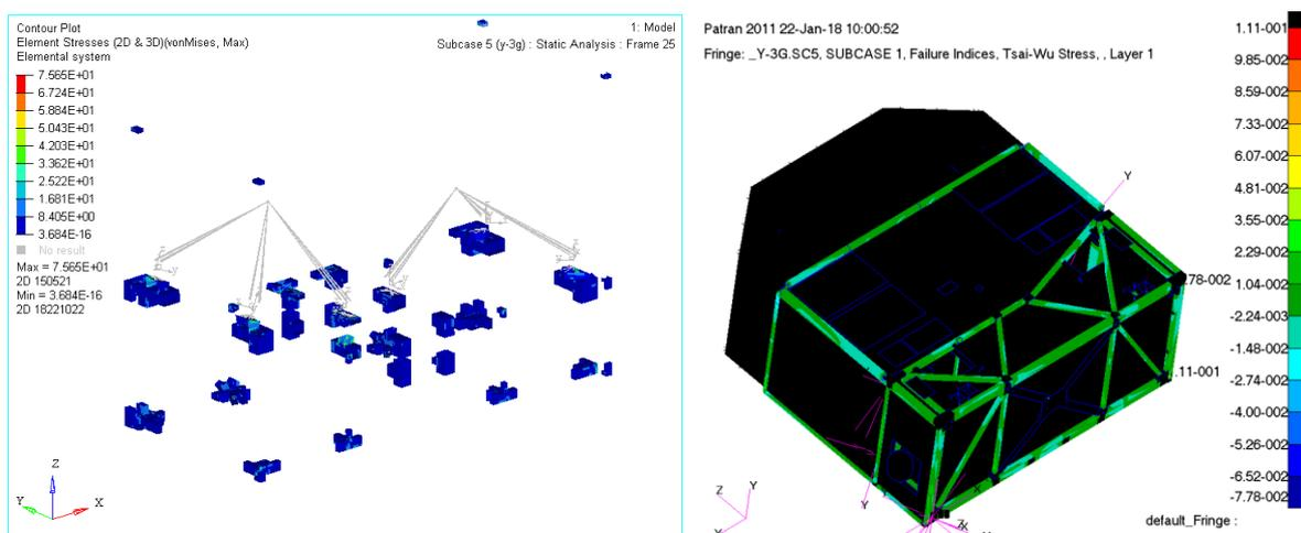
**Figure 7.** Cloud chart of stress distribution in titanium alloy joints and composite material failure indices by the Tsai-Wu criterion
