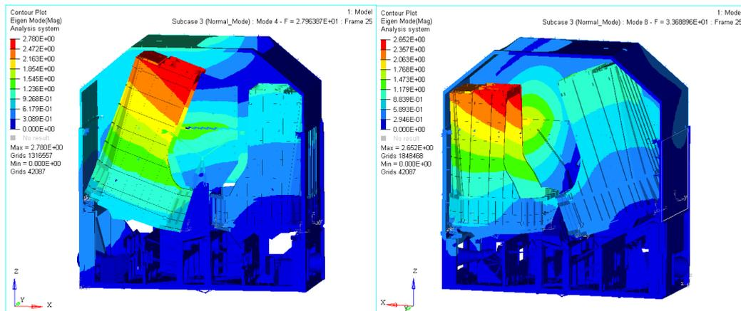
a) third-order mode front camera at 28Hz    b) fourth-order mode rear camera at 33.5Hz
