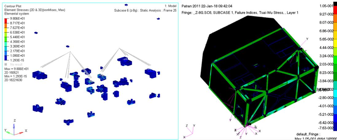
Figure 8. Cloud chart of stress distribution in titanium alloy joints and composite material failure indices by the Tsai-Wu criterion
