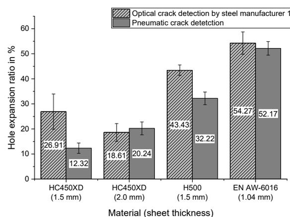
**Figure 2.** Comparison of hole expansion ratios during stop of the test, using optical and pneumatic method for a dual-phase steel sensitive to edge cracks (a) and for other car body materials (b).
