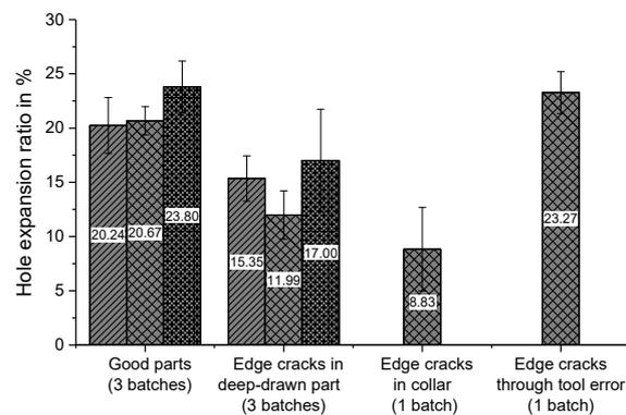
**Figure 3.** Investigation of the influence of various parameters on the hole expansion with pneumatic stop method for the dual-phase steel HC450 XD 1.5 mm (a-c), investigation of the edge crack sensitivity of good and bad batches of the dual-phase steel HC450XD 2.0 mm with pneumatic crack detection (d).
