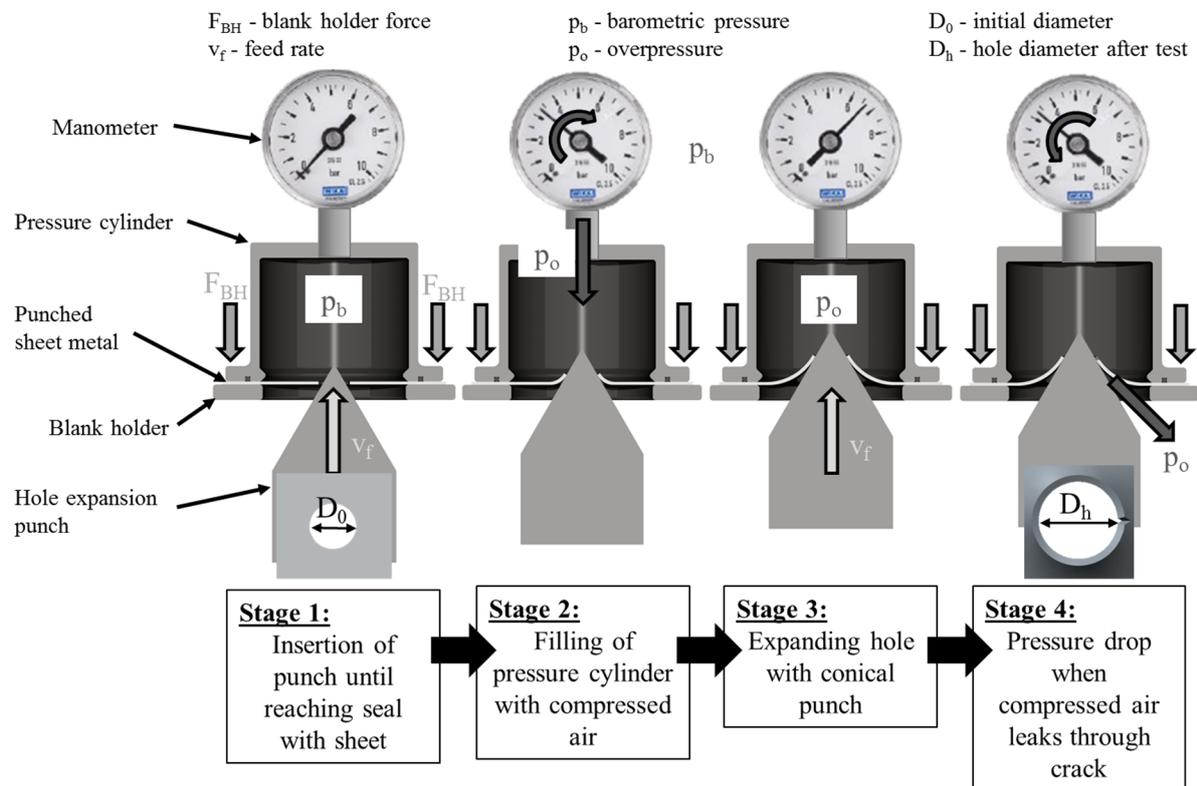
**Figure 1.** Schematic structure and sequence of the hole expansion test with pneumatic crack detection.
