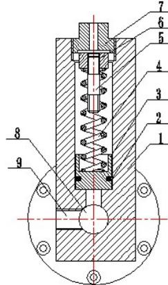
1 - energy accumulator cavity; 2 - Glyd ring®; 3 - piston; 4 - spring; 5 - screw; 6 - cushion block; 7 - plug; 8 - oil inlet; 9 - pressure sensor installation hole
