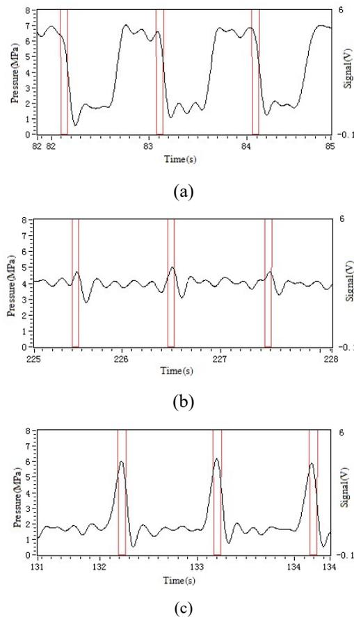
**Fig. 4** Effect of off-pulse position on modulation pressure
