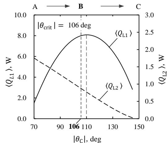
**Figure 4.** Cooling capacity vs  $\theta_C$  curve of a Stirling/pulse tube hybrid cooler Sage model
