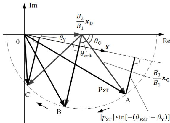
**Figure 3.** A phasor diagram of the Stirling/pulse tube hybrid cooler with various  $\theta_C$ .
