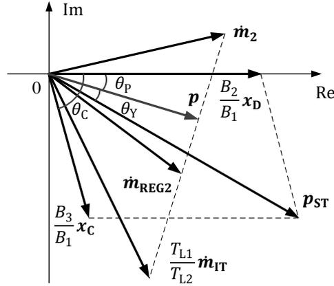
**Figure 2.** A typical phasor diagram of the Stirling/pulse tube hybrid cooler.
