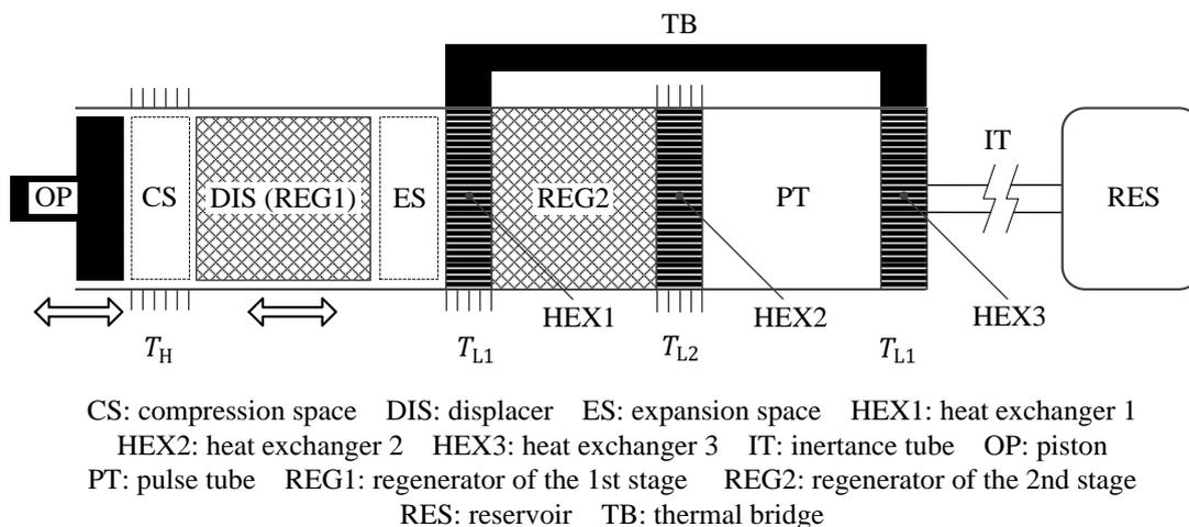
**Figure 1.** A diagram of a Stirling/pulse tube hybrid cooler with cold inertance tube.
