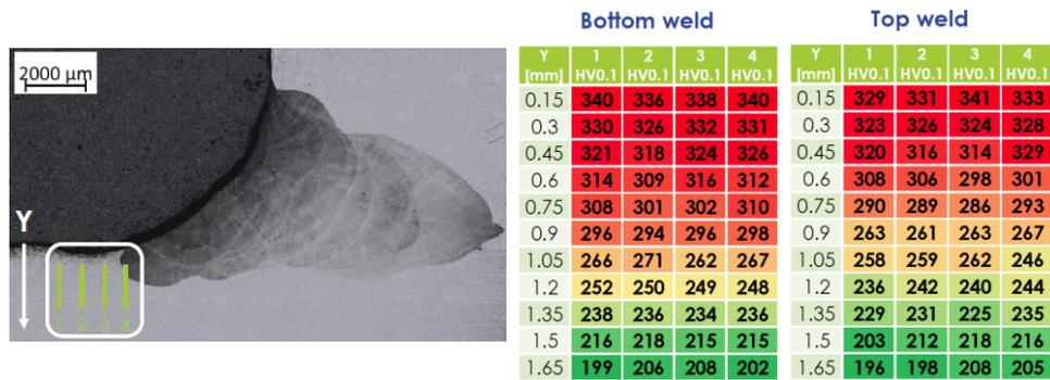
**Figure 6.** Results of microhardness testing on shot peened welds. Left, schematic representation of the four microhardness lines measured under the weld toe in a cross cut along the horizontal axis of the conductor. Right: matrix of the measured microhardness values. The vertical distance between indentations along the Y-axis is 150  $\mu\text{m}$  (Y represents the distance from the peened surface), while the distance between two adjacent columns is 1 mm
