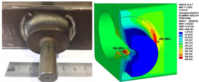
**Figure 1.** Left: view of a CS helium inlet. The contour of the weld between the conductor jacket and the nozzle is shape-optimized and locally processed by USP (metal shining portions). As shown by the finite element model (right), the stresses are the highest at the weld toe around the longitudinal axis. The second region of stress concentration is at the bottom of the internal diameter hole
