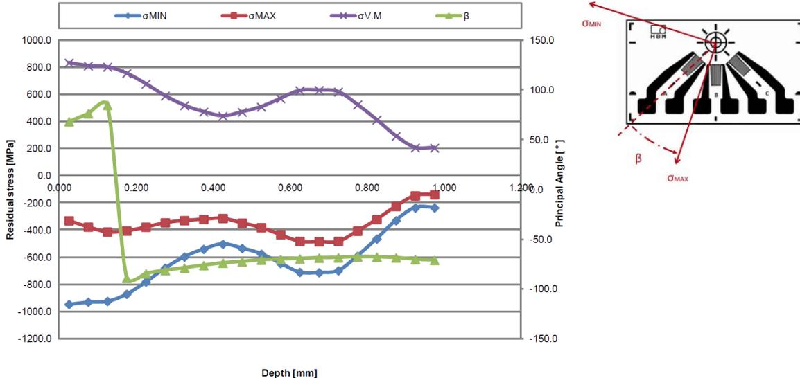
**Figure 4.** Residual stress in function of the thickness for the top inlet weld of sample “2P”. On the x-axis, the depth is measured from the weld toe.  $\sigma_{\text{MIN}}$  ( $\sigma_{\text{MAX}}$ ) is the minimum (maximum) principal stress,  $\sigma_{\text{V.M}}$  is the equivalent Von Mises stress,  $\beta$  is the principal angle referred (and positioned in the correct quadrant) according to the convention of ASTM E837 (method CCW for rosette type B)
