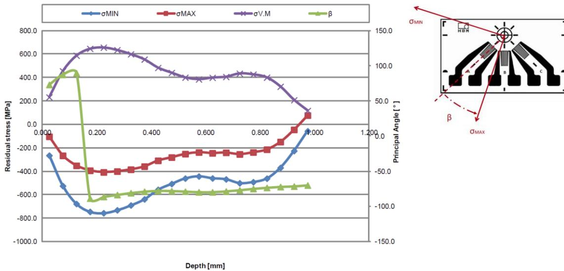
**Figure 5.** Residual stress in function of the thickness for the bottom inlet weld of the same sample
