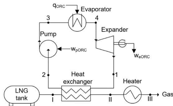
Figure 1. Scheme diagram of analysed ORC system.
