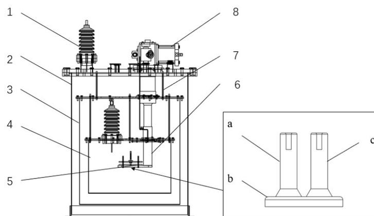
**Figure 1.** Schematic of the sample chamber. (1) feedthrough; (2) vacuum chamber; (3) the first thermal radiation shield; (4) the second radiation shield; (5) electrodes; (7) mechanical support and (8) GM cryocooler; (a) cathode; (b) copper plate and (c) anode
