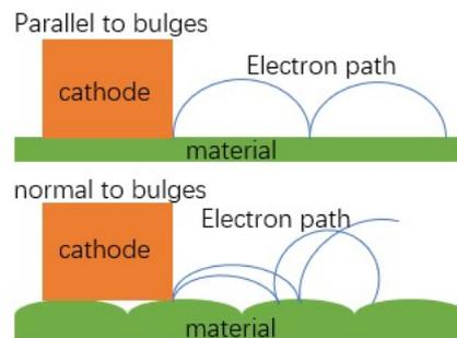
**Figure 4.** Flashover process in different orientations
