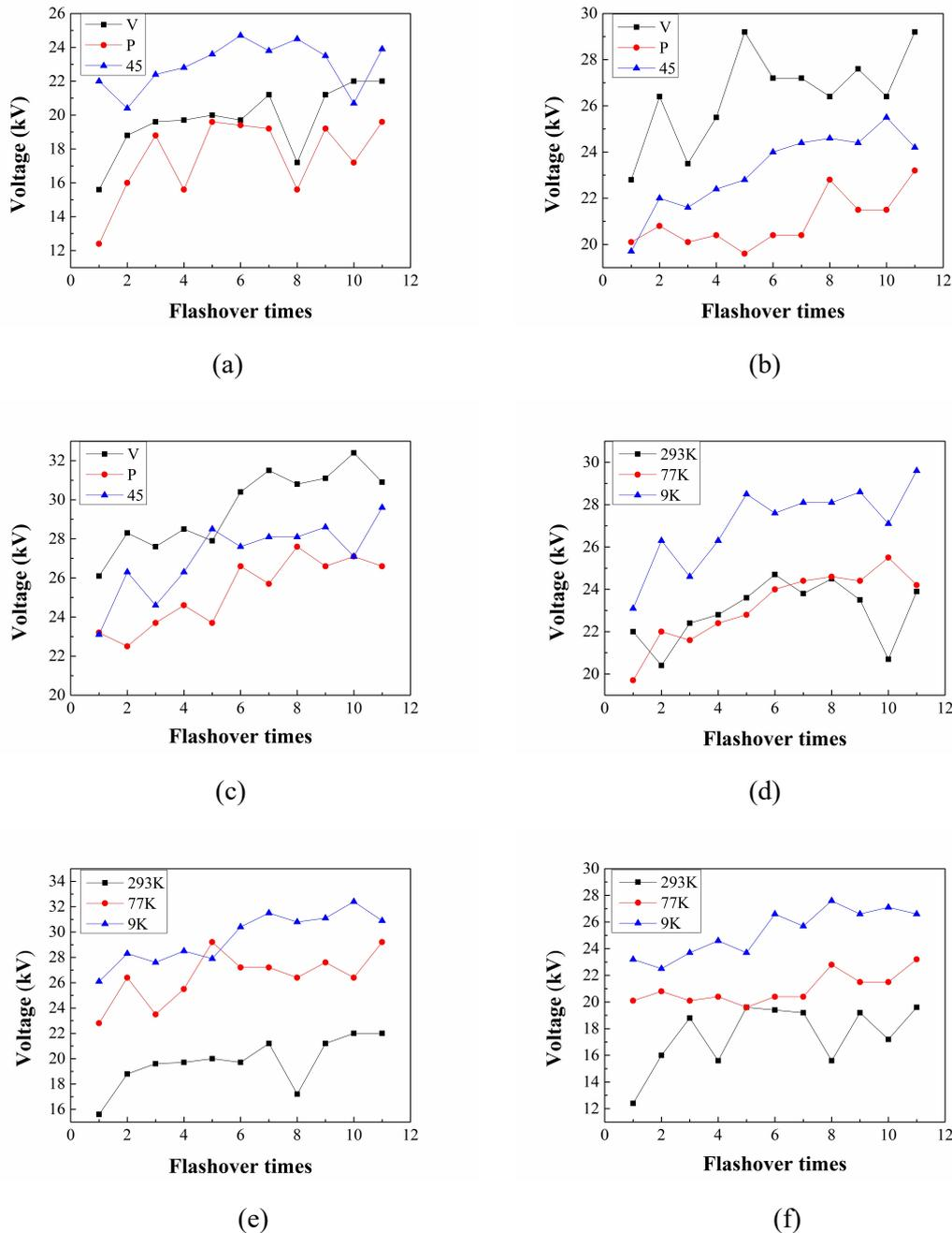
**Figure 3.** Flashover strength of the G-11 with different orientations and temperatures: (a) Flashover voltages at 293K, (b) Flashover voltages at 77K, (c) Flashover voltages at 9K, (d) Flashover voltages in 45-degree angle, (e) Flashover voltages in vertical and (f) Flashover voltages in parallel
